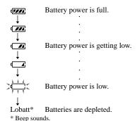
To keep the original battery capacity for a long time, charge the batteries only when they are completely depleted.
